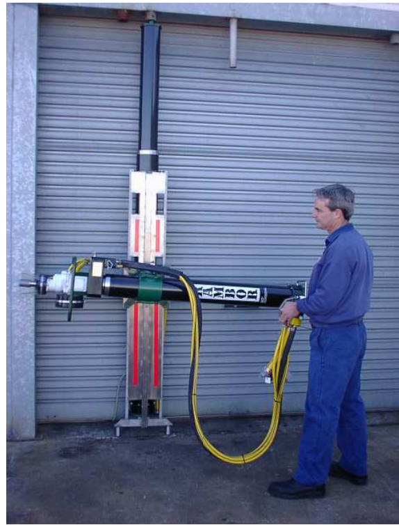
Photo shows the RDR2 with: Two Stage / Double Acting Longwall Face Drill with 1.3 or 1.7 metre Stroke
